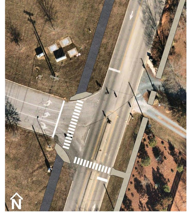
Aerial conceptual rendering of Project Int-06, showing the proposed marked crossing at the existing signalized intersection with high visibility marked crosswalks, conversion of the raised median to a refuge island, and connection to the sidewalk extension and SUP.
