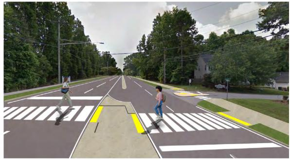
Project Int-43 conceptual rendering from person-level perspective showing the inclusion of the controlled pedestrian crossing at the Kingston Dr intersection that includes high visibility marked crosswalks and a pedestrian refuge island.
